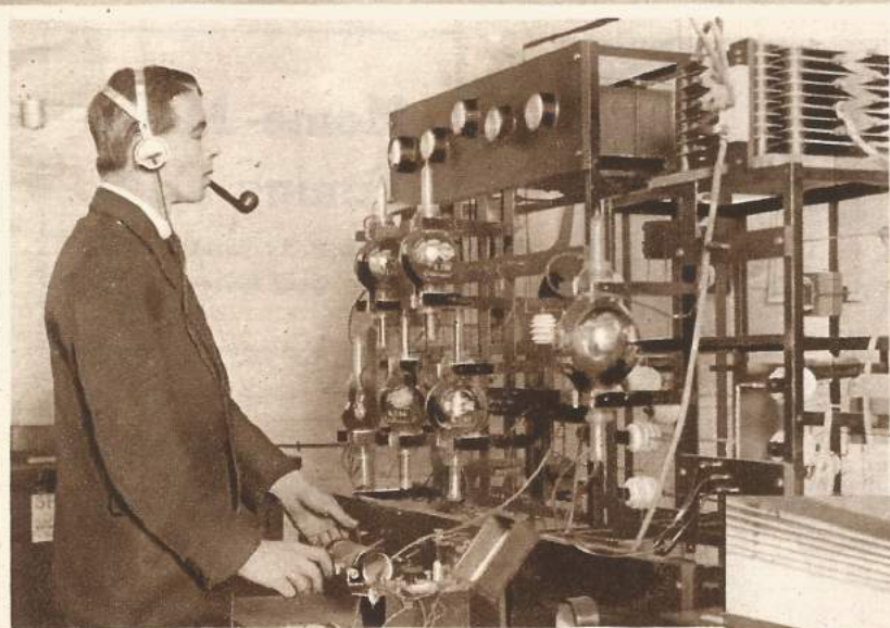
Mr. P. H. Cook, Assistant Engineer at the Hull Relay Station, adjusting the transmitter. This photograph gives a good idea of the size of valves used.
