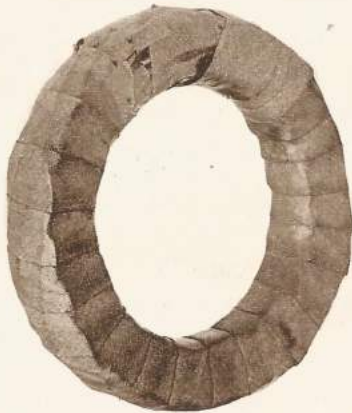
Fig. 7.—The end of the tape is secured with Chatterton's compound.
