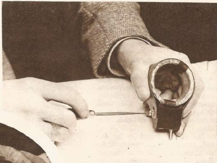
Fig. 8.—The coil may be attached to the plug by means of a band and two screws.
